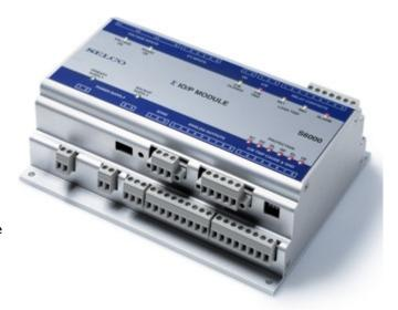
The S6000 measures the voltages across all three phases as well as the current running through each phase. The voltage and current signals are digitally sampled by the built-in signal processor and converted to true RMS values. The S6000 will continuously do real-time calculations of voltage, current, frequency, active/reactive power, VA, power factor etc. The S6000 can connect to generators with or without neutral.
